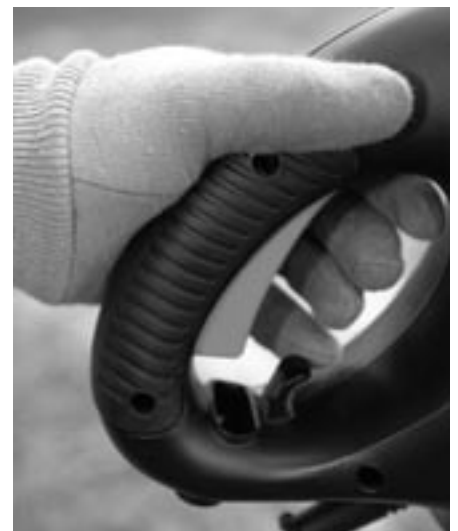
Figure 3-8: Releasing trigger switch to stop trimmer
